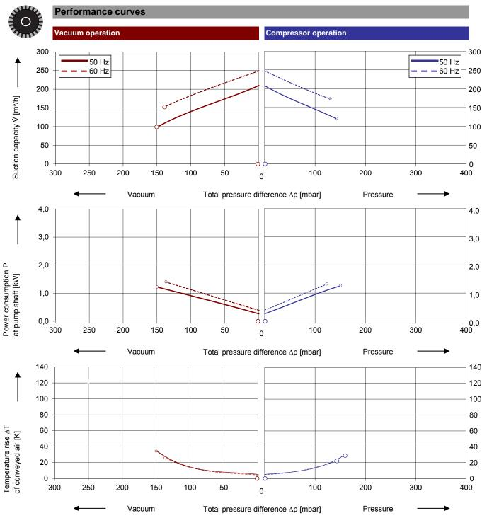
The performance curves are based on air at a temperature of 15  $^{\circ}\text{C}$  and an atmospheric pressure of 1013 mbar with a tolerance of  $\pm$  10 %. The total pressure differences are valid for suction and ambient temperature up to 25  $^{\circ}\text{C}$ . For other conditions please get in touch with us.
